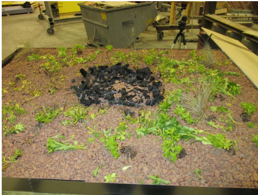
Photo No. 7 Burning Brand Post Test (Typical)
