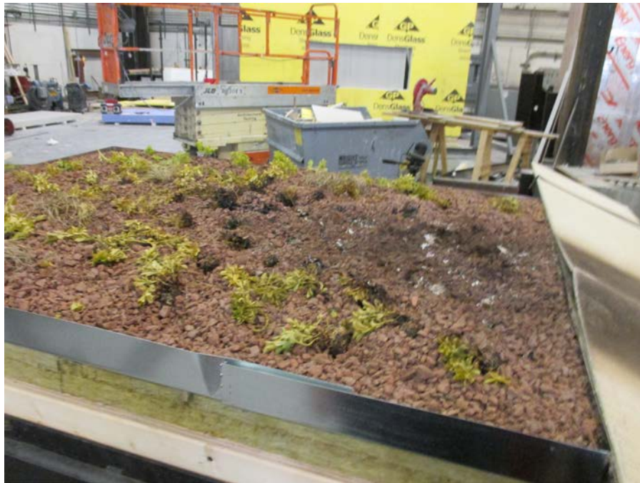
Photo No. 5 Intermittent Flame Post Test (Typical)
