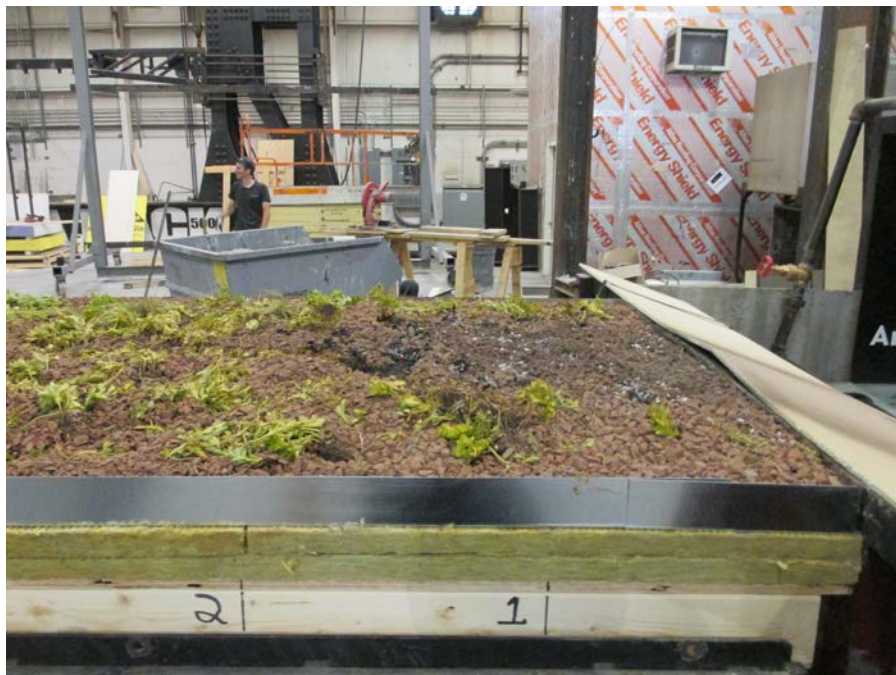
Photo No. 6 Spread of Flame Post Test (Typical)
